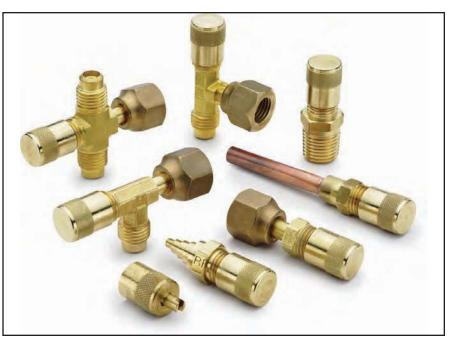
Designed to offer convenient low cost access ports for refrigeration service. All fittings feature 1/4" SAE male flare access ports and are furnished with a finger tight quick seal cap. Access valves with pipe connections have internal ODS solder cups.
