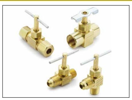
Needle valves have metal-to-metal seats with fine thread screwdown. Brass construction with specially formulated low temperature seal which remains elastic to temperature as low  $-40^{\circ}$ F.
