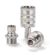
Brass coupling with no valve for applications with liquids in the pressure range up to 35 bar. The couplings are corrosion resistant. The system stands out for a high flow with minimal pressure drop.
