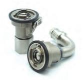
Eaton's FD83 is designed for electronics cooling applications where full flow, fluid compatibility and safety are essential. The FD83 identical halves include two interlock features to eliminate spills and ensure maximum safety. Valves cannot be opened until the coupling halves are mated and coupling halves cannot be disconnected until both halves are closed.
