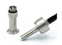
Eaton's Blindmate QD (BQD) is a non-spill coupling used for water cooling systems on IT racks. This coupling is connected blindly when the operator inserts the blade into the rack. The locking mechanism is then deported on the rack system, the coupling does not have its own locking mechanism.
